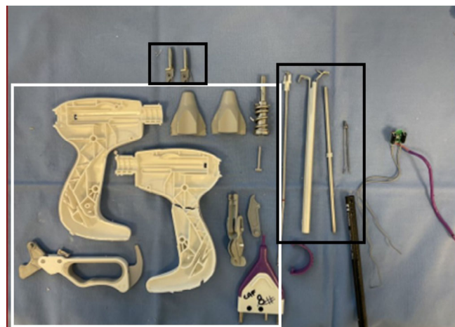
FIGURE 2 Photograph of a vessel sealing device (Ligasure Atlas, Medtronic Covidien) used in the current study after being completely disassembled into individual pieces and separated by the pieces associated with the handpiece (pieces within the white square) and the pieces related to the jaws of the device (pieces within the black rectangles). Each individual piece was then thoroughly assessed for the presence or absence of biologic debris following use in live clinical dogs for an assigned number of splenectomies.
